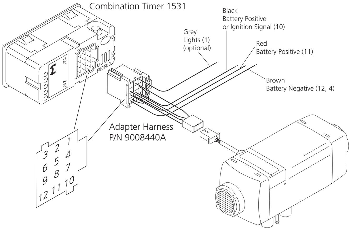
Figure 14: Schematic Connection of the Combination Timer Model 1531
