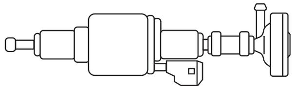
**Figure 10: Fuel Metering Pump DP 30.2/3 (with Damper)**
