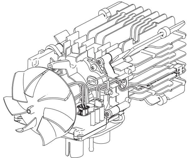
**Figure 2: Air Top 2000 ST Air Heater without Casing**
