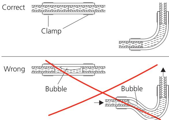
Figure 19: Pipe/Hose connections
