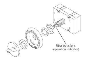
Figure 25: Control element (rheostat switch)
