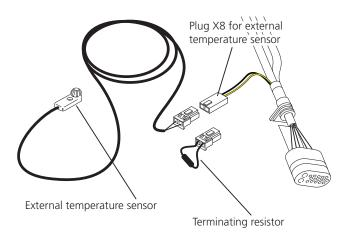
Figure 28: External Temperature Sensor
