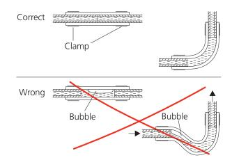
Figure 19: Pipe/Hose connections
