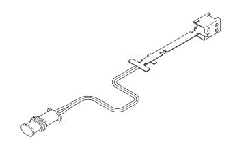
Figure 9: Overheating Sensor
