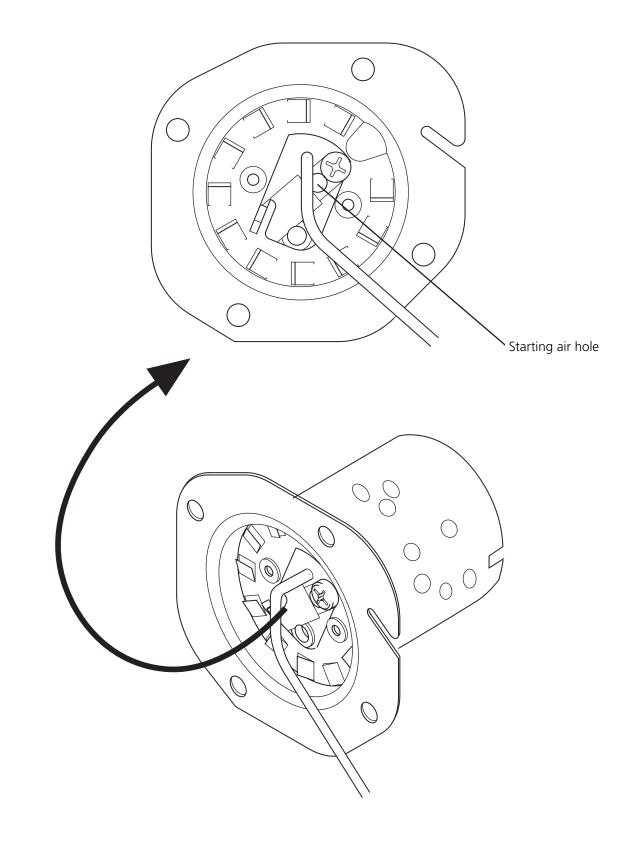
Figure 32: Starting air hole in burner insert
