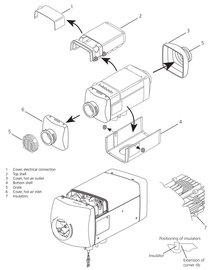
Figure 29: Remove / Fit the Casing Parts
