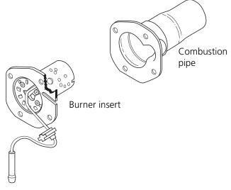
Figure 5: Burner Insert with Combustion Pipe
