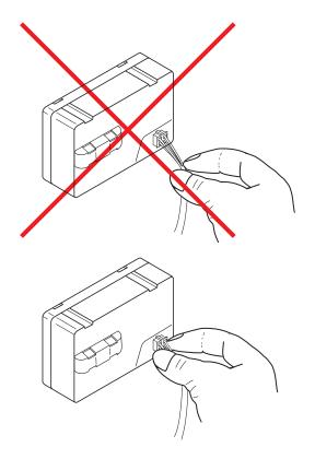
Figure 26: Disconnecting the plug
