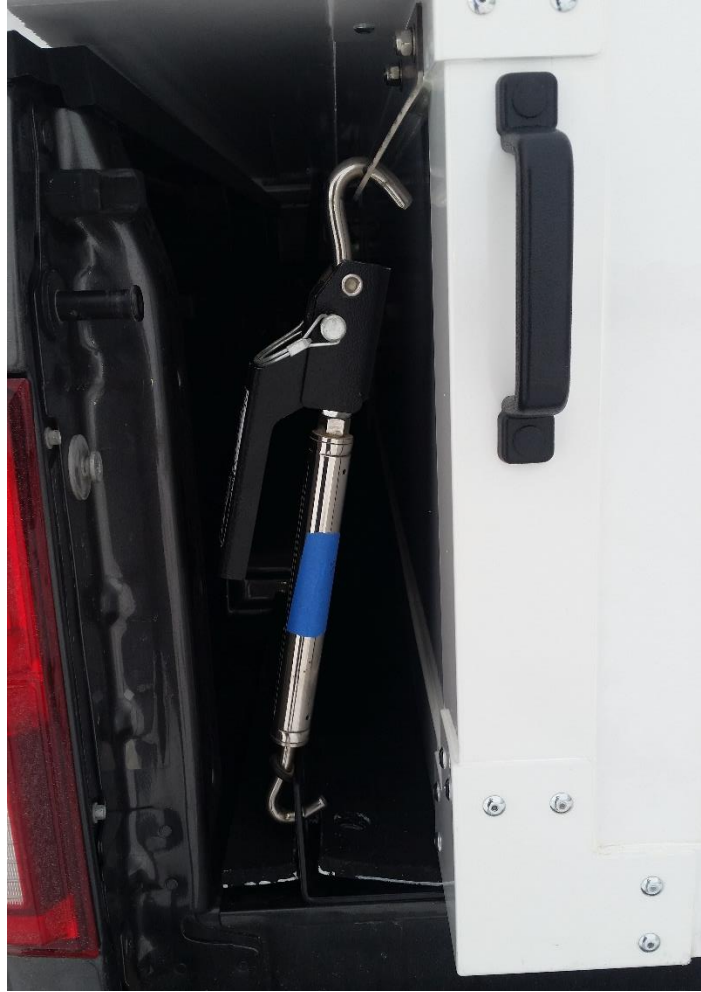
Tie down fully closed and safety pin installed.
