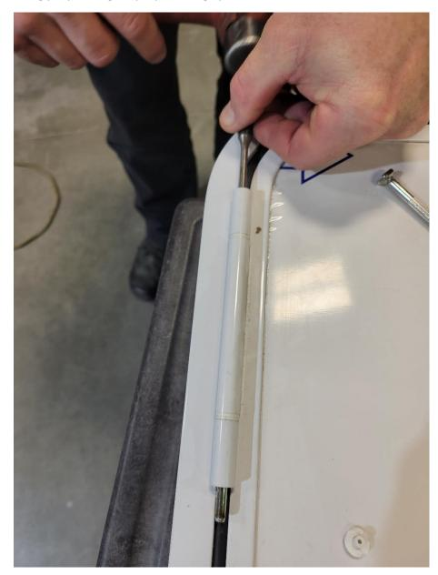
• With a long pin punch, gently tap the hinge pin out
