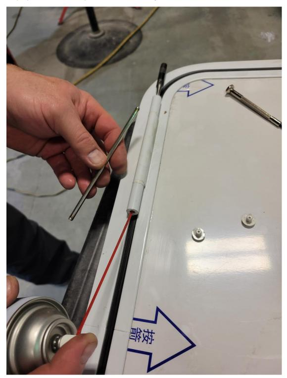
• Spray lubricant into the pin bore, Fluid Film is a great lubricant for this as it is wax based
