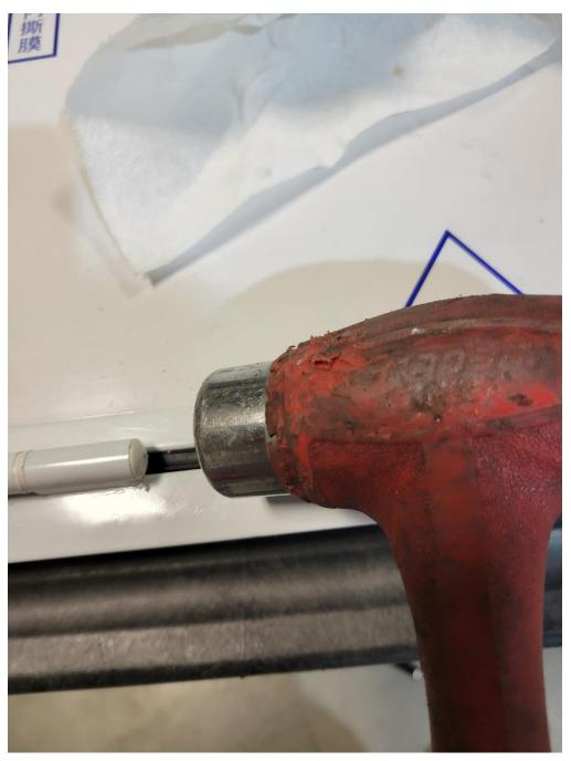
• The plugs have a light press fit, they are also glued from the factory, the gluing process requires the hinge to be completely dry and oil free, this is also what causes the issue of hinge seizure. We will be looking for an alternative plug for the pin bore in case the originals get damaged or won't stay in place after lubricating.
