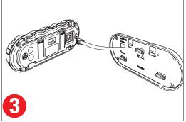
Feed the Remote Monitor cable through the hole and connect it to the Remote Monitor.
