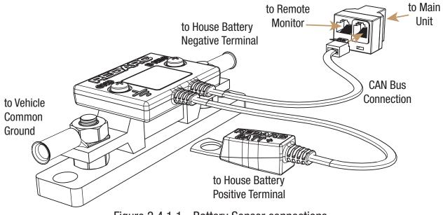
Figure 2.4.1.1 - Battery Sensor connections
