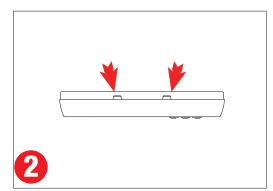
The locking tabs can be accessed through holes on the top of the backing plate when installed.
