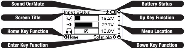
Figure 3.2.1 - The LCD Display
