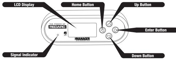
Figure 3.1.1 - The Remote Monitor
