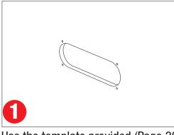
Use the template provided (Page 36) to mark the position and drill and cut the mounting holes into the wall.
