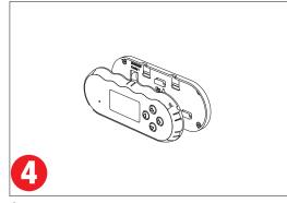
Clip the Inner Assembly into the Back Plate.
