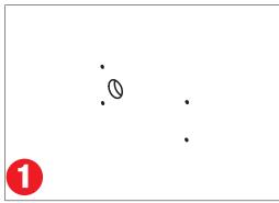
Use the template provided (Page 36) to mark the position and drill and cut the mounting holes into the wall.
