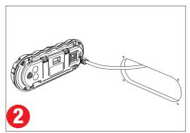
Feed the Remote Monitor cable through the hole and connect it to the Remote Monitor.
