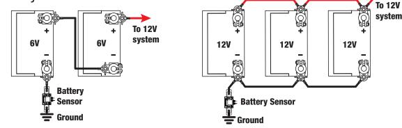
Figure 2.5.1 - Batteries in Series.
