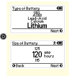
The Type of Battery screen allows the user to indicate the type of battery being charged by The Manager30. This setting will affect the charge profile that The Manager30 uses to charge the battery so it is important to select the correct battery type. Once you are happy with your selection move on to the Size of Battery screen.
