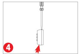
When the screwdriver is in a vertical position, gently push upwards on the bottom of the Remote Assembly to unlock tab. Repeat 3 & 4 for 2<sup>nd</sup> tab.
