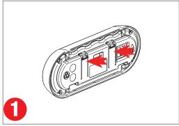
The locking tabs on the back of the Inner Assembly need to be unclipped from the Back Plate.
