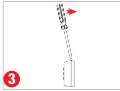
Insert a flat-head screwdriver at a slight angle towards the front of the Remote Monitor and push back to depress the locking tabs.
