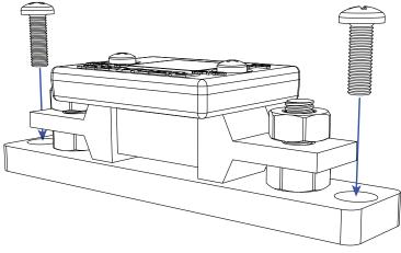
Figure 2.2.3.1 - Mounting the Battery Sensor
