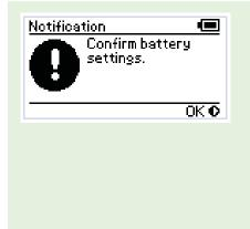
The second and most important step required for initial setup is Battery Type and Size selection. Please refer to the battery manufacturers specification sheet for Size(AH) and Type specifications. If you are unsure of the type of your battery please select the Gel setting. Should power to the Battery Sensor be removed at any time, the unit will revert to the Gel setting and prompt the user to input their Battery Type again. The Battery Size setting will be retained in memory.
