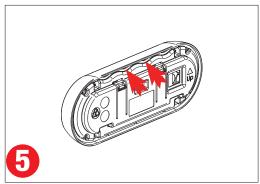
Slide fingers between the Front Face and the Inner Assembly in positions marked above and carefully pull back towards the front of the Remote Monitor.
