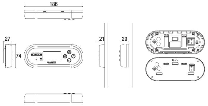
Figure 1.4.2 - Remote Monitor Dimensions
