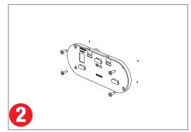
Attach the Back Plate to the wall using 4 suitably sized countersunk screws.
