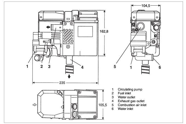
Fig. 301: Heater Dimensions
