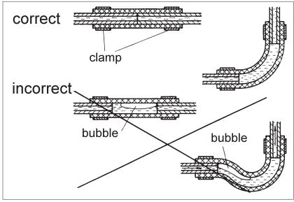
Fig. 407: Fuel Line Connection
