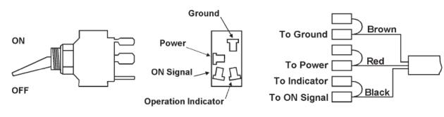
Fig. 408: On/Off Toggle Switch
