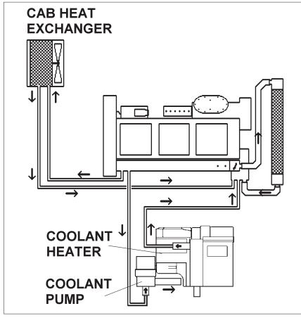
Fig. 403: Engine Block Preheating
