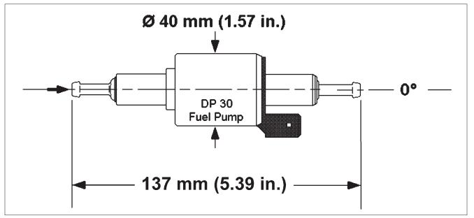
Fig. 302: Fuel Pump Dimensions
