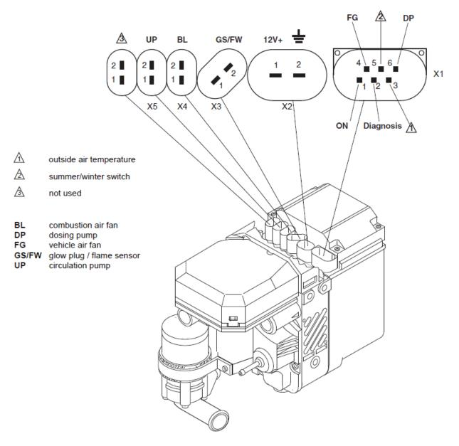
Fig. 411 Control Unit Connector Pin Assignment (Thermo Top C)
