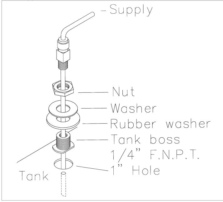
Fig. 406: Fuel Standpipe
