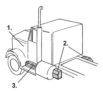
CAUTION! Do not mount the heater directly to the engine! Heavy, constant vibration produced by the engine may interfere with the proper operation of the heater and lead to heater component damage.
