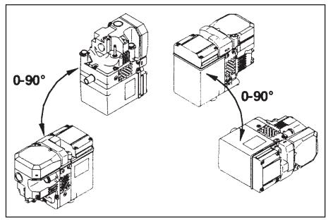
Fig. 402: Permissible Heater Installation Positions
